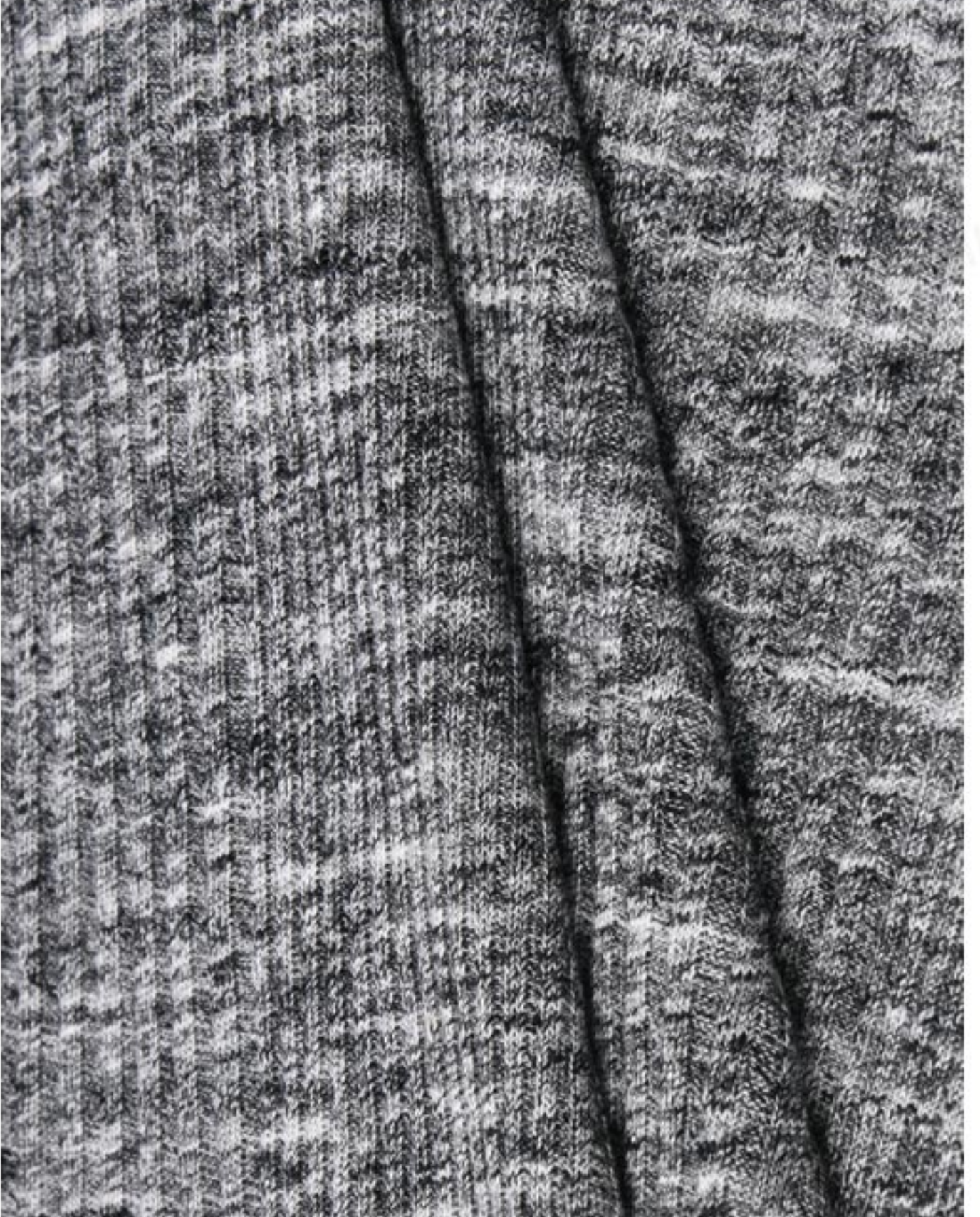
22NW-2122 Stripped Rib Spec: 65% polyester, 35% cotton, 21S, 160GSM, 132cm
