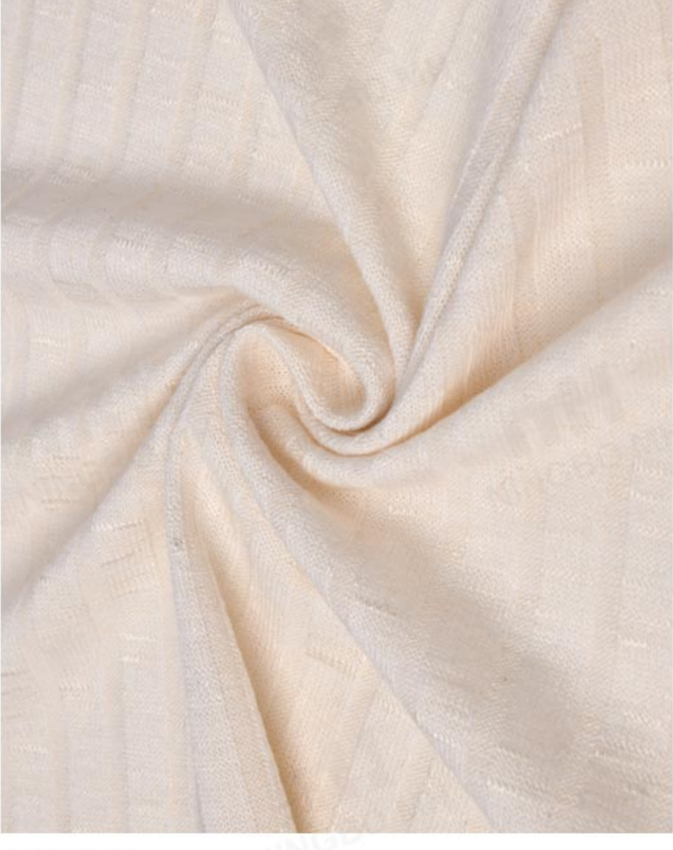
22NW-2118 9*4 Slub Rib Spec: 53% Rayon 43% Polyester 4% Spandex, 30S Rayon slub + 30S Polyester + 30D Spandex, 220GSM, 152cm
