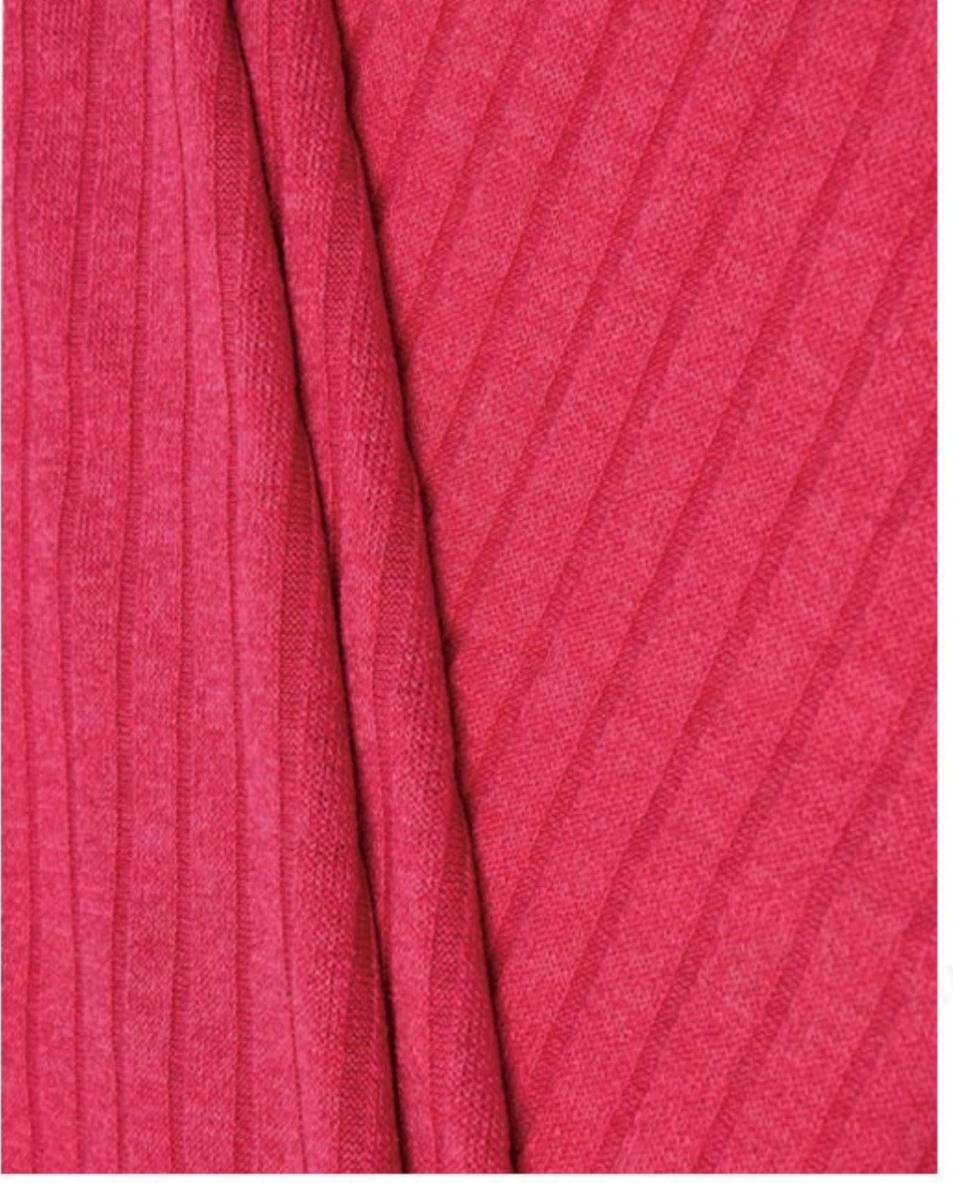
22NW-2116 8*4 Rib Spec: 95% Polyester 5% Spandex, 30S Polyester+ 240D DTY+30D Spandex, 205GSM, 148cm
